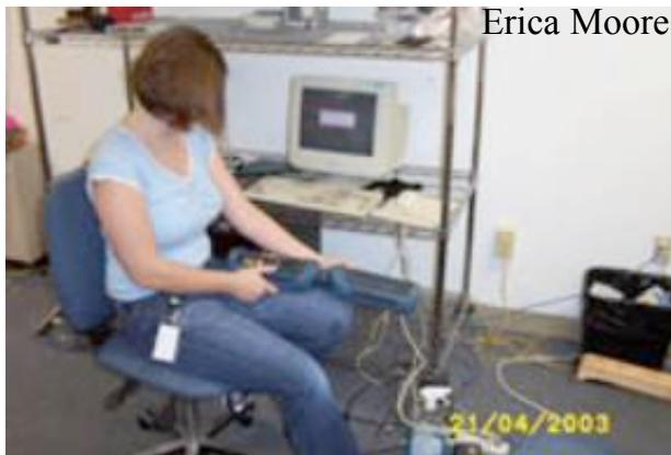
Charging the wire tester (tests for attenuation, etc.)
